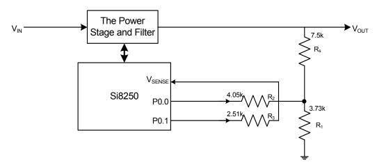
Figure 8. The Example Voltage Sense Circuit
