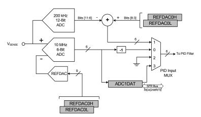
Figure 1. ADC1 Block Diagram
