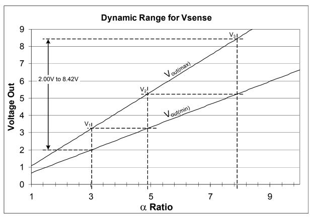
Figure 6. Graphical Determination of the  $\alpha$  Ratios
