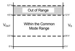
Figure 4. Output Voltage Limit
