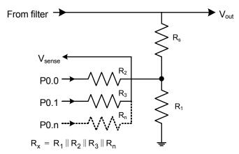
Figure 5. Feedback with Common Mode Compensation
