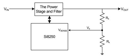
Figure 3. Resistor Divider
