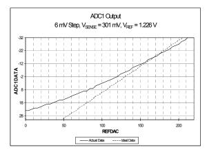
Figure 2. ADC1 Results Below the Common Mode Specification
